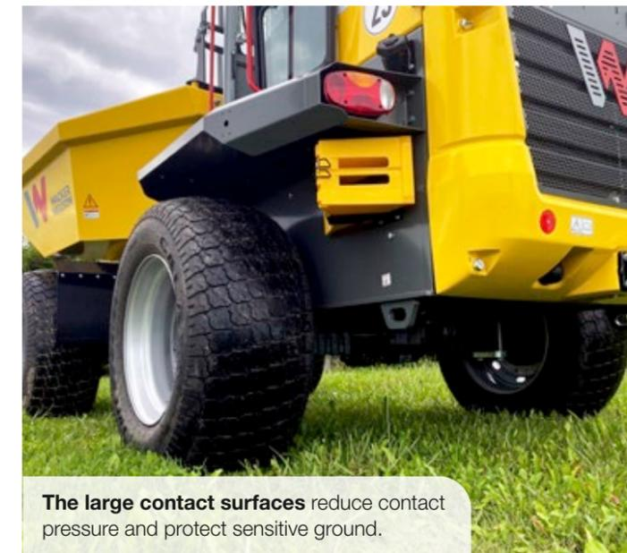
The large contact surfaces reduce contact pressure and protect sensitive ground.
