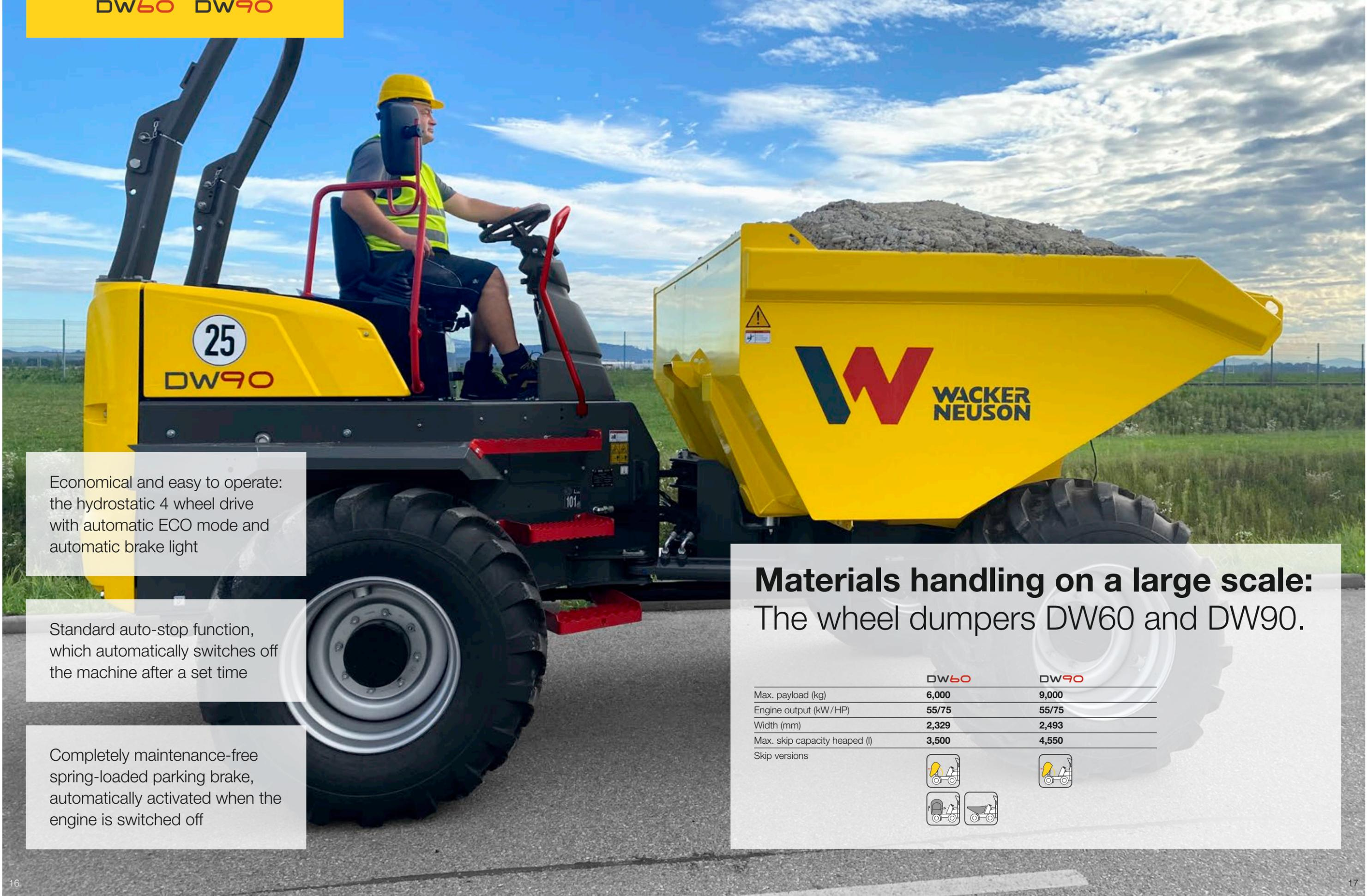
Economical and easy to operate: the hydrostatic 4 wheel drive with automatic ECO mode and automatic brake light
