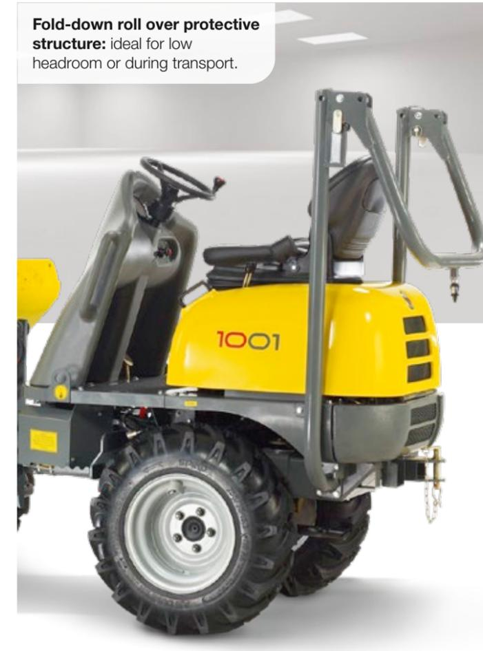
**Simple operation, low wear:** the hydrostatic twin-lock 4-wheel drive saves time and money
