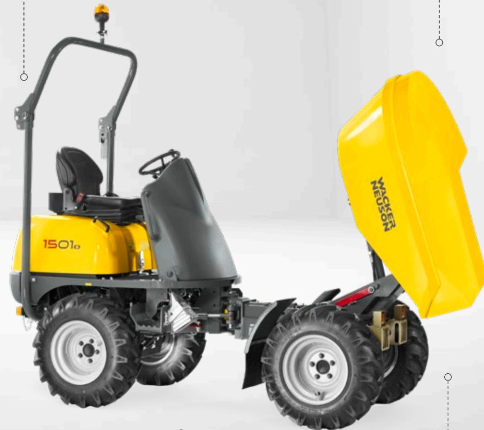
**Reversing alarm and side mirrors** for optimal all-round visibility and more safety on the construction site
