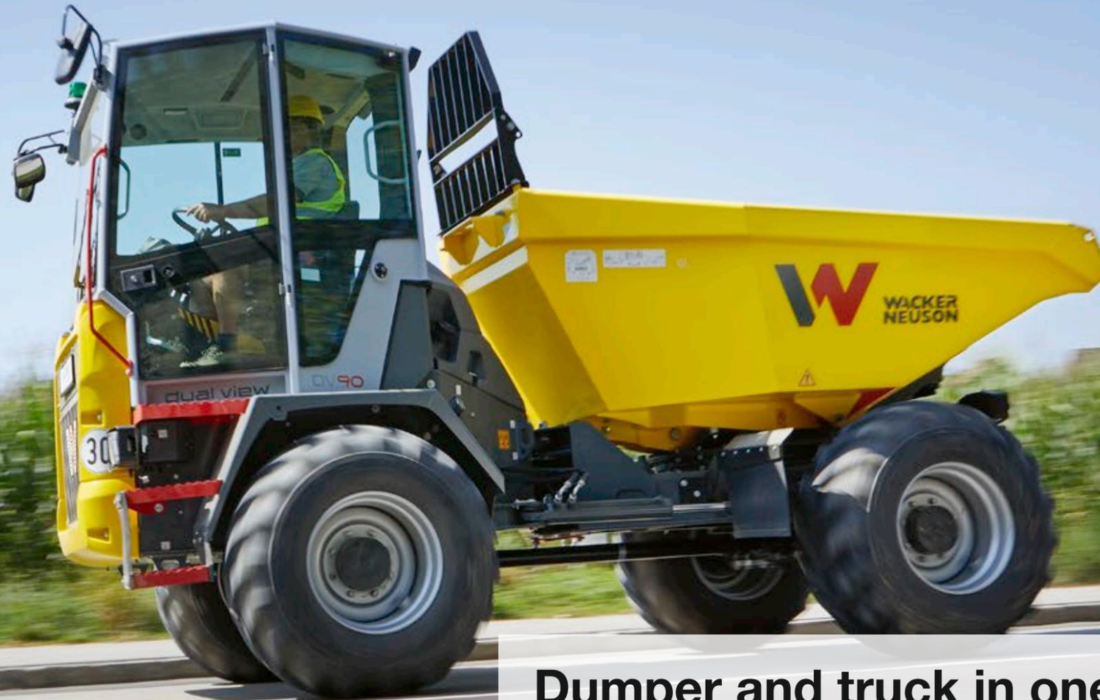
Innovative Dual View concept: 180-degree rotatable operator's seat offers the ideal view when loading and driving
