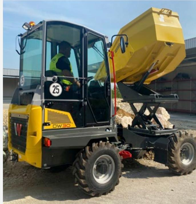
**The built-in auto-stop automatic function** automatically switches off the machine when not in use, thus saving operation and maintenance costs.
