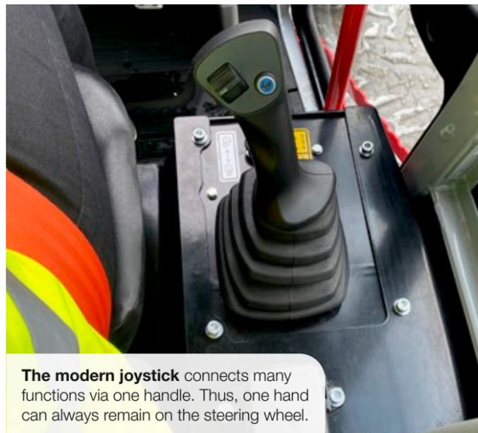
The modern joystick connects many functions via one handle. Thus, one hand can always remain on the steering wheel.
